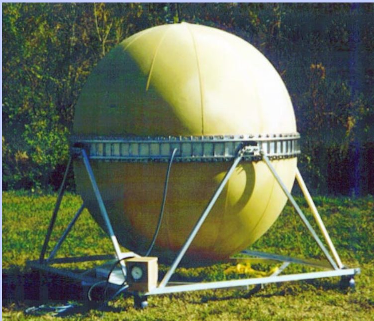
Kevlar pressure vessel undergoing pressure testing.
